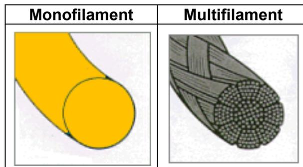
With very few exceptions screen printing mesh is made from monofilament, multifilament tends to be used as filtration mesh, which is closely allied to screen mesh.
