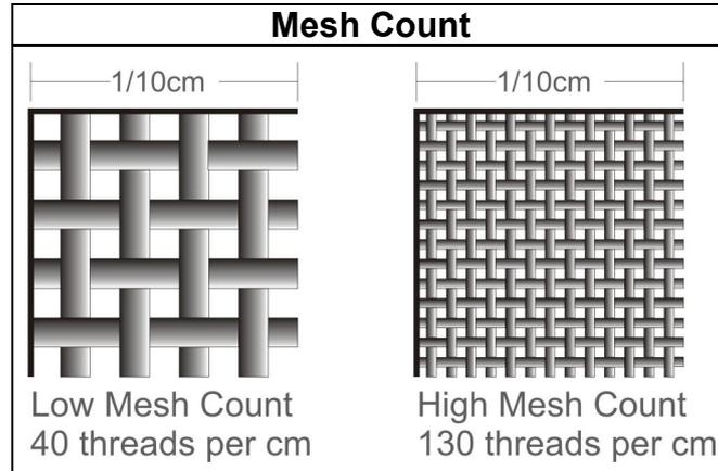
For a given mesh count there can be more than one thread diameter. For example a 90 t.p.cm mesh can have thread diameters of 40, 49 and 50 microns. This in turn will affect mesh openings and thickness of the mesh.
