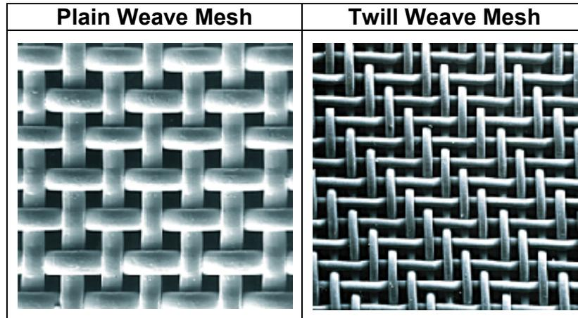
Twill weave meshes are available in some mesh types and normally for mesh counts above 120 t.p.cm. If you do use them their performance will be different to a plain weave of the same mesh count. The twill weave has a tendency to put more ink down but the contact between the knuckles of the mesh and the substrate can interfere with the spread of ink in the image area, particularly on fine lines. You must be aware of the characteristics and always specify precisely what you want.
