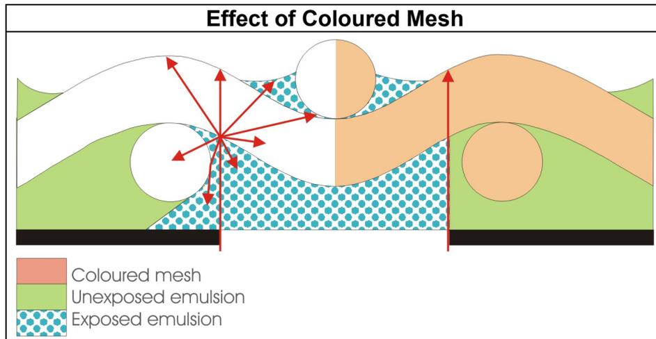
Mesh colour is the final issue. Yellow and Orange are preferable to white if fine detail is important. The colouring reduces light scatter through the threads. White is really only recommended when exposing with direct projection where the lower level of Ultra Violet dose could be unacceptably reduced by yellow or orange coloured mesh.
