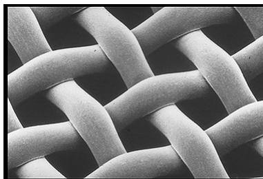
Many attempts have been made to replace woven mesh as the basis of the screen printing process, only in the electronics industry where stainless steel masks are used for depositing solder paste has this proved successful even here the mesh has not been replaced it has been removed altogether.
