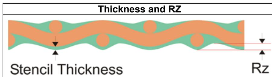
Should edge definition of the image be critical an Rz meter to measure the roughness of the print side of the stencil will also be necessary.
