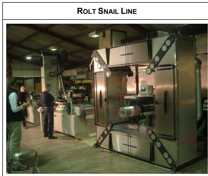
A typical innovative solution where space was an issue was the Rolt “Snail Line” Here the dryer was formed into a square and the take off was place in the centre of the square. In so doing this reduced the length and height of the line substantially.
