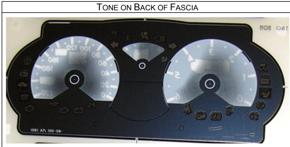
To check that the colours and levels produced are to specification the output from the illuminated fascia has then to be measured with a spectrophotometer. During production densities of filters have been checked with a densitometer.
