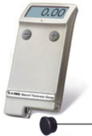
The snap measurement probe was developed by SPTF in co-operation with KIWO it uses their thickness gauge instrument to give accurate snap measurement. The probe can be placed in different positions on the stencil to ensure that the snap distance is consistent.
