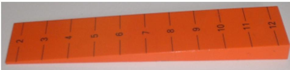
Slid underneath the frame or clamping rails the Snap Wedge is a simple means of checking distance from machine bed. Straightforward calculation gives snap height.
