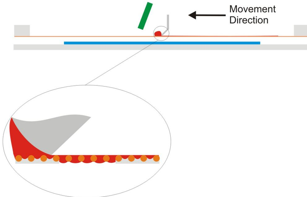
Setting the squeegee is about it being parallel with the substrate with sufficient pressure applied to bring the stencil into contact with the substrate and cause the ink to flow through the mesh. The measurements that are required are the set angle, the amount it protrudes from the squeegee holder and the actual squeegee hardness. If any of these are left to chance then control of the process is compromised.
