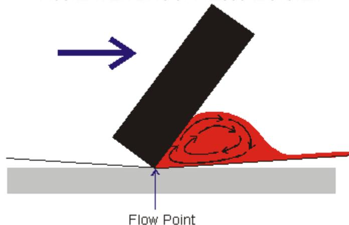
As the angle gets smaller the amount of ink increases up to the maximum that the mesh will permit. For the sake of simplicity the point on the squeegee at which the ink is caused to flow through the mesh, openings should be known as the “Flow Point”.
