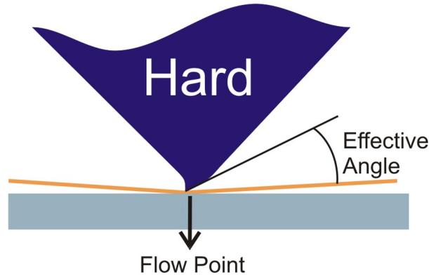
Less distortion of tip with a hard squeegee, large effective angle.
