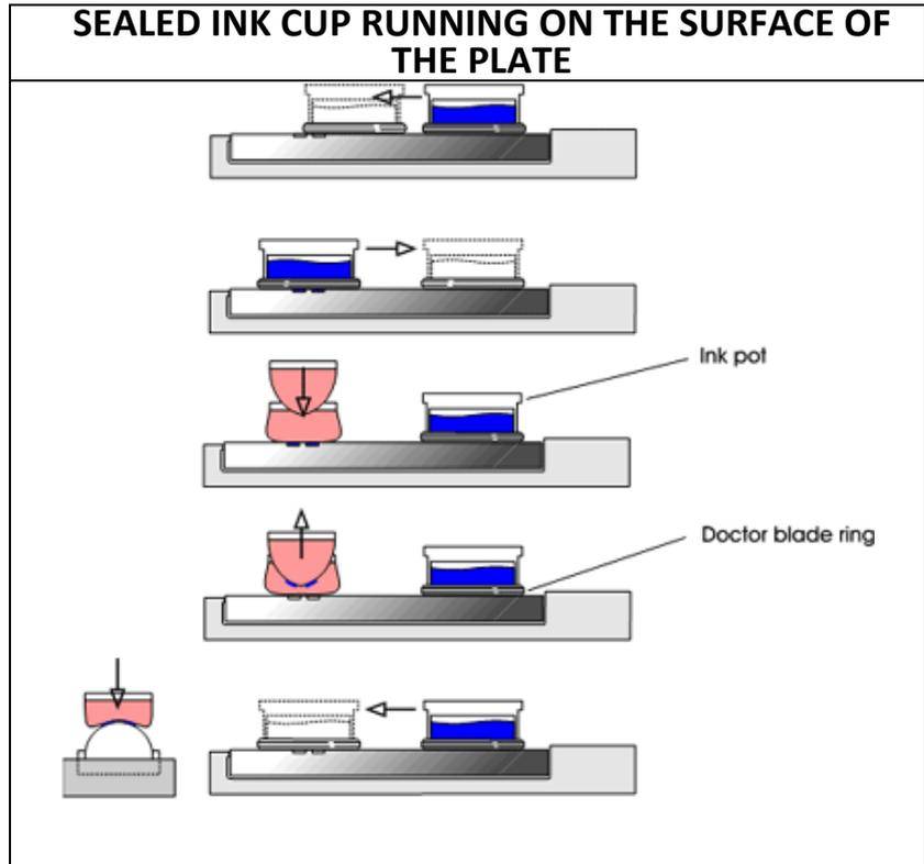
The answer can come as a surprise. £500 is not at all unusual. Fortunately, if the damage to the cup is very slight it is possible to carefully hone the contact surface on a fine carborundum stone. Some cups can be re-machined at a quarter of the replacement costs. This all means the cups must be handled very carefully. The plate has to be twice the size of a conventional plate for a given image.
