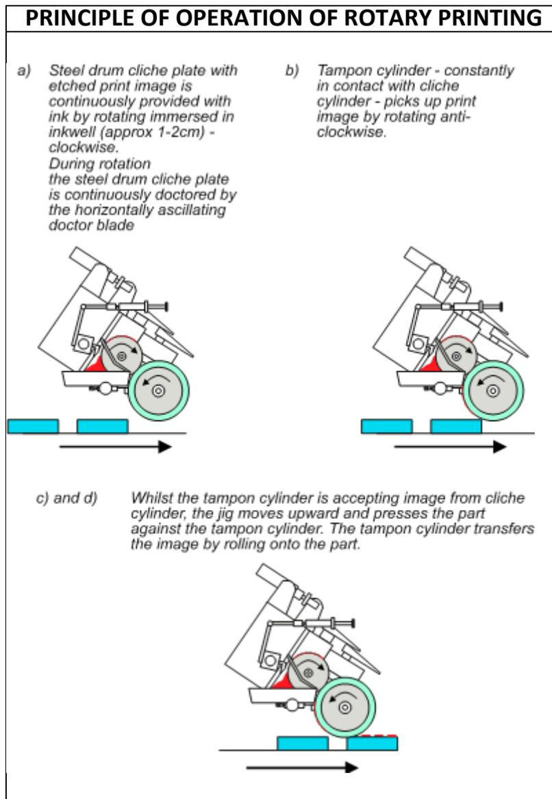
There are alternatives to the steel printing cylinders. Steel foil plates or even photopolymers can be mounted onto a modified cylinder. Their effectiveness is debatable as the pressure on the doctor blade causes them to wear fairly quickly. Although the steel cylinders are by no means cheap the investment is paid back by reduced down time.
