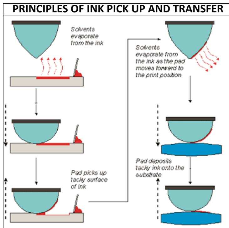
Evaporation of solvents is a key mechanism of the process. Controlling the rate of evaporation to suit the application is one of the factors in selecting a machine.
