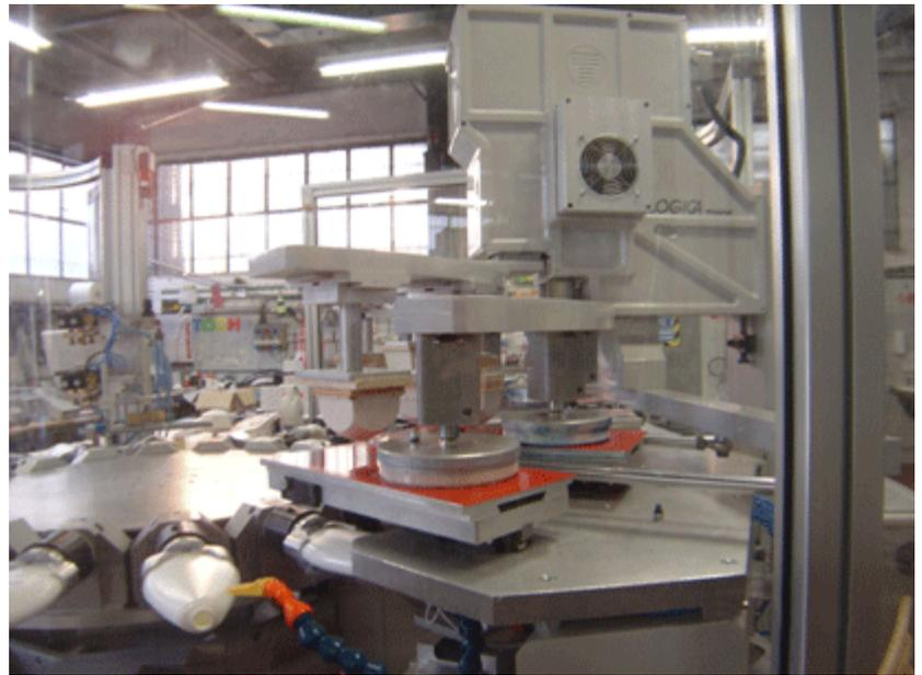
Even Tampoprint, for years the doyen of pad printing machinery manufacturers has available their Sealed Ink Cup 60/90 machine that is an evolution of the Hermetic closed cup machine that for some time was the fastest pad printer available, capable of print speeds of 5400 per hour. The Sealed Ink Cup 60/90 reaches 3500 provides a high quality print within its 90 mm closed cup.
